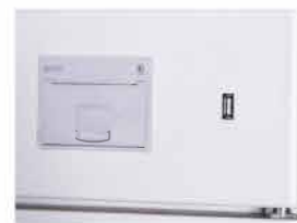
Thermal printer and USB interface
